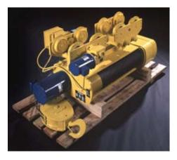
Class C Moderate Service (CMAA Definition) - the crane will handle loads which average 50% of the rated capacity with 5 to 10 lifts per hour, averaging 15 feet, not over 50% of the lifts at rated capacity. Class D Heavy Service (CMAA Definition) - loads approaching 50% of the rated capacity will be handled constantly during the working period. High speeds are desirable for this type of service with 10 to 20 lifts per hour averaging 15 feet, not over 65% of the lifts at rated capacity.
