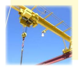
Both chain and wire rope hoists are rated H-4 (heavy duty) or H-3 (moderate duty). Duty ratings are a better indicator of hoist durability than hoist type (chain or wire rope). Both types of hoist use similar motors, brakes and controls. The main difference between electric chain hoists and wire rope hoists is in the design of the lifting mechanism. Be sure to request an H-4 rating on either hoist type to ensure long life and low maintenance.
